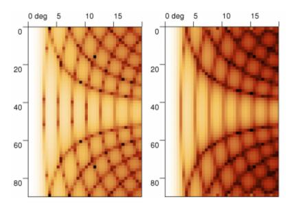
Comparison can be even better done on single profile across the direction of diffraction pattern as shown below. Note the effect of limited angular resolution of the calculation which can be one of reasons of small differences (besides limited NFFF integration area and other numerical errors).
