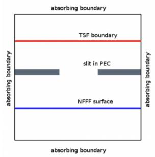
Near-to-far field transformation (NFFF) integrated from plane behind the aperture is used to calculate far field radiation pattern. Preserving both TSF source and NFFF integration plane close to metal plane helps to minimize influence of finite plane wave and metal plane size.
