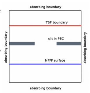
Near-to-far field transformation (NFFF) integrated from plane behind the aperture is used to calculate
