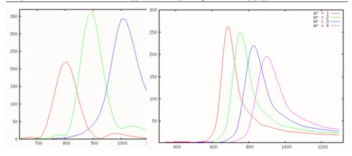
Similar results can be obtained for two triangular metallic objects used as nanoantenna (see the simulation snapshot in bottom right figure). Here a spectral dependence of the field enhancement between the objects is shown for two different sizes of the whole system (I: total length, g: gap width) for wavelengths from 300 to 1300 nm.
