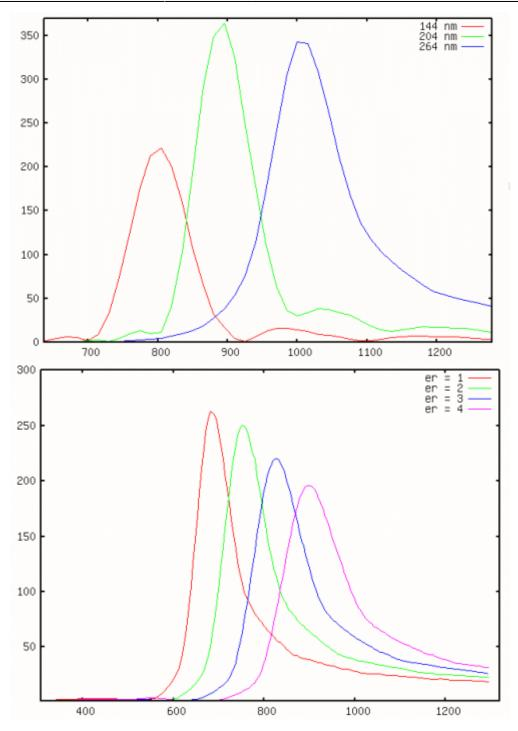
Similar results can be obtained for two triangular metallic objects used as nanoantenna (see the simulation snapshot in the right figure). Here a spectral dependence of the field enhancement between the objects is shown for two different sizes of the whole system (I: total length, g: gap width) for wavelengths from 300 to 1300 nm.
