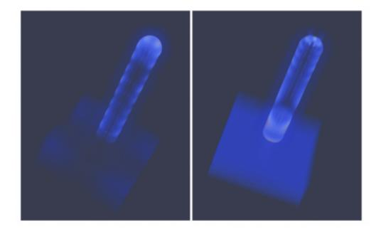
Similar calculation can be performed for any wavelength within range of our optical data (and reasonable ratio between wavelength and voxel spacing). Here a set of simulation snapshots for different wavelengths is shown for single column structure illuminated from bottom:
