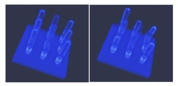
Geometrical model can be made even more complex, e.g. by adding scanning probe microscope tip to the structure. This geometry is similar to what we use in photoconductive AFM measurements. After adding simple tetrahedral tip we get this snapshot and volume absorption (tip only sketched on absorption image).
