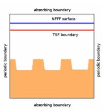
values of electric and magnetic properties are loaded for full volume (an alternative would be to load Gwyddion height field using vector material approach, or to construct totally synthetic vector data input based on primitive geometric entities).
