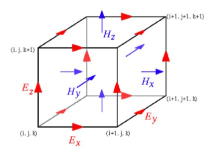
The benefit of this scheme is that we can easily draw a electric field loop around a concrete component of the magnetic field and vice versa. This simplifies the implementation of rotations in the Maxwell equations significantly.
