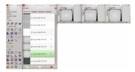
Note that in this example we have clicked on  $Data\ Process \rightarrow Presentation \rightarrow Logscale$  for every displayed output to see the data in better scale. We can see that in different cross-sections of the computational space there is a wave similar to a dipole output.
