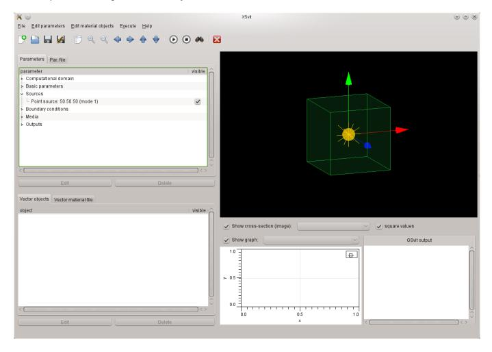
Next we will add **point and image outputs**. This is done by menu entry *Edit parameters->Add point output* and *Edit parameters->Add image output* that again open dialogues for specifying how often (parameter "skip") and which component should be output. Point output is collected from a single point within computational volume and is stored into a text file. Image output comes to general
