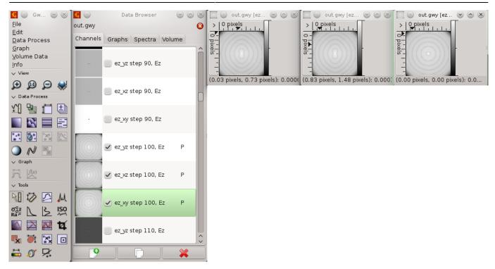
Note that in this example we have clicked on *Data Process->Presentation->Logscale* for every displayed output to see the data in better scale. We can see that in different cross-sections of the computational space there is a wave similar to a dipole output.
