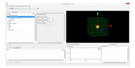
It is reasonable to save your parameter file at this stage using <i>File→Save</i> command. We can do it also later, just before running computation, however doing it right now will set the current directory and other input/output files set later can be referred to it (instead of using absolute path). Moreover, by saving parameter file we also set default directory for temporary files (e.g. generated sources), which is also important.
