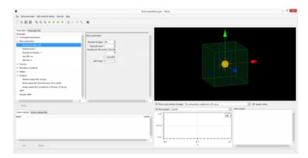
Finally we need to save the parameter file if we haven't done it at beginning, as since now we worked only with a temporary file or at least modified file (it is important to save it always before running computation which is not done automatically). This is done by  $File \rightarrow Save$  command as usual. Then we can **start the computation** clicking on the arrow in the toolbar or using  $Execute \rightarrow Run$  menu command.
