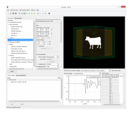
In documentation related to FDTD calculations via GSvit, which lists all the possible options and algorithms, both the parameter file setup and XSvit based setup is always mentioned. There are also sample parameter files to be directly used for further modifications, either via XSvit or a text editor.
